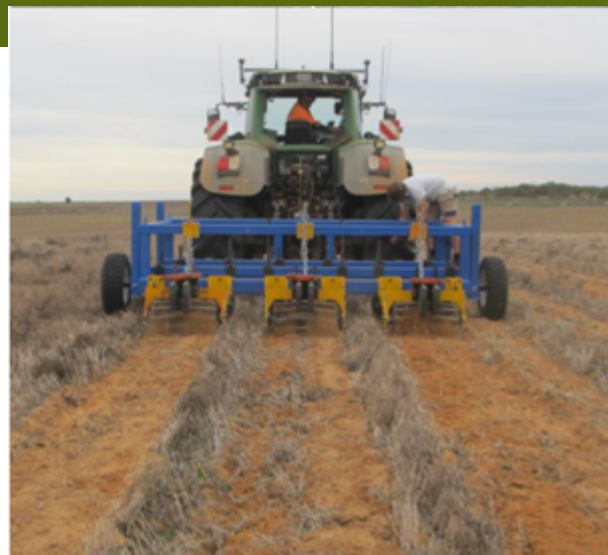
Strip ripping leaving strips of standing stubble. Photo: UniSA
