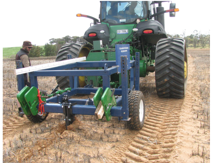
Figure 2: Collaborative research ripper frame supplied to the University of South Australia by Agrowplow-Davimac and combined with a 3-point linkage force measuring frame to evaluate the performance of a selection of ripper tine technologies in deep sand.
